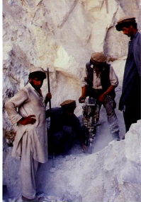
Figure 6. Mining at Jegdalek is small scale. The only mechanized equipment consists of a few pneumatic hand drills. Photo by Gary Bowersox.
