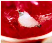
Figure 14. Translucent white masses were frequently encountered at the surface of the polished corundums in this study. These remnants of the marble host rock were typically composed of calcite, sometimes with apatite and/or margarite. Photomicrograph by Christopher P. Smith, magnified 25 \times .
