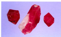
Figure 11. These three ruby specimens show the appearance of corundum crystals from Jegdalek. The two smaller crystals are typical, whereas the longer crystal in the middle has relatively large pyramidal faces. Two sets of twinning lines parallel to r ( 10\bar{1}1 ) are also visible in the largest crystal, which measures 2.0 cm long. Photo by Maha DeMaggio.
